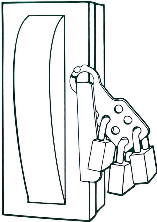
Figure 19-5. Lockout hasp on an electrical control panel that provides a method for applying a lock (lockout) to the panel during maintenance or repair to ensure that the equipment is not energized until the work has been completed. The control panel should also be tagged (tagout) with a label indicating that work is being performed. Workers should be provided with individually keyed locks, and only the worker who applied the lock should remove it. (Source: Occupational Safety and Health Administration. Concepts and techniques of machine safeguarding. Washington, DC: OSHA, 1980.)
