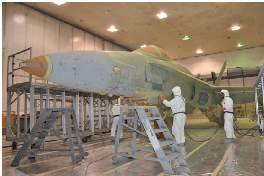
Figure 2. Navy artisans (sprayers and hosemen) applying primer during F-18 strike fighter aircraft paint finishing operations.
