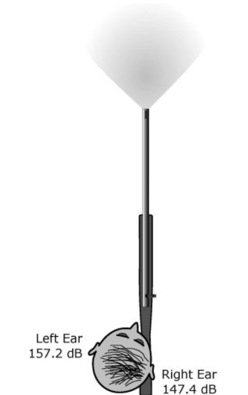
Figure 3 Illustration of head-shadow effect contrasting sound pressure levels measured for each ear for a right-handed rifle or shotgun shooter.
