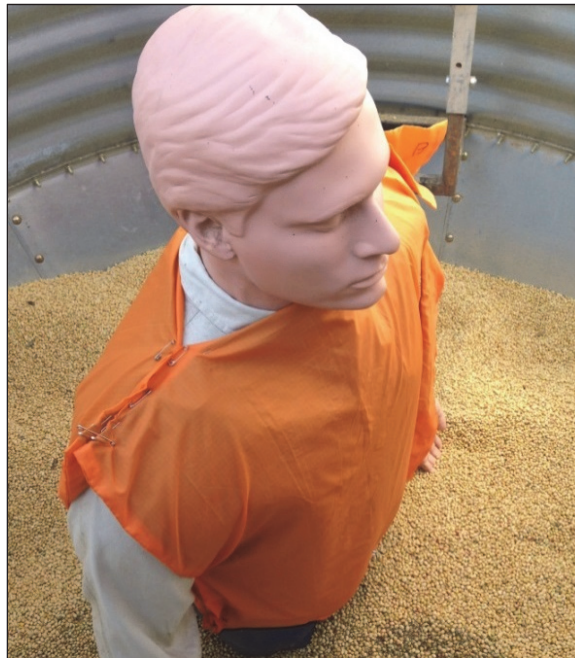
Figure 2. Rescue manikin outfitted with sensor mats prior to testing in soybeans.
