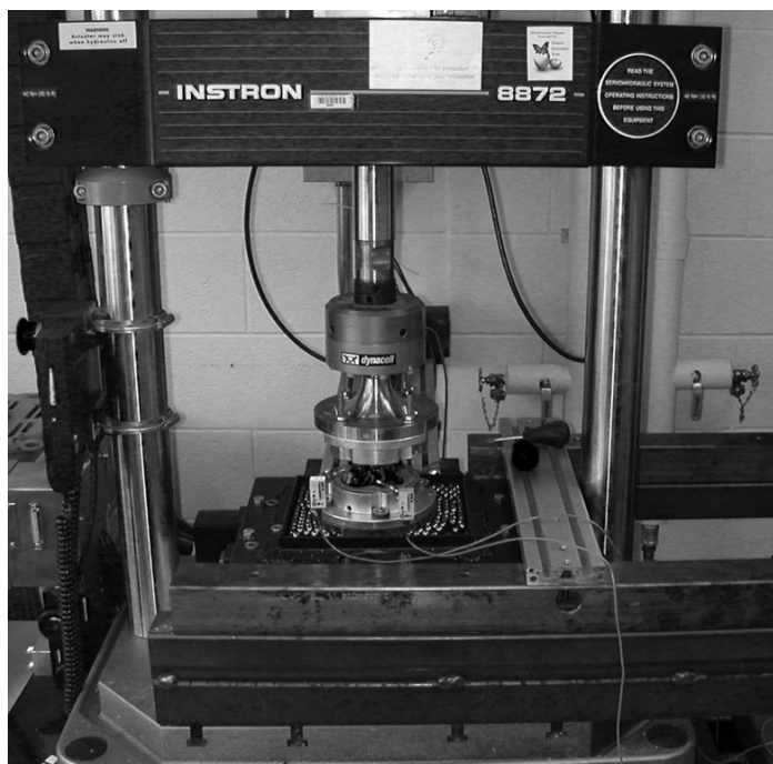
Figure 1: Biomechanical test setup for cyclic compression.
