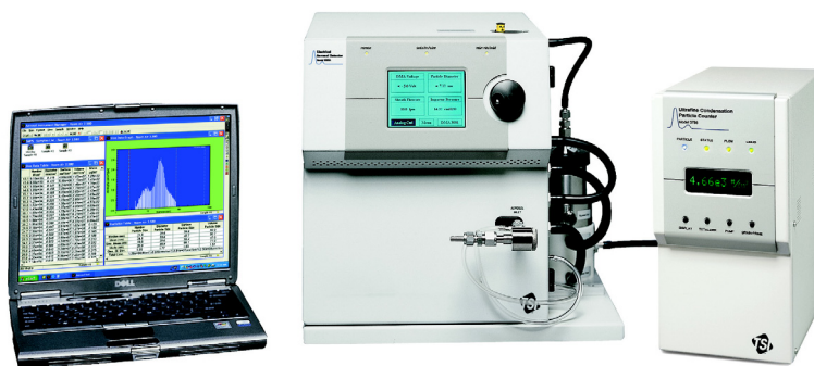
Fig. 5.4. An example instrument for measuring the electrical mobility particle size distribution of airborne NPs is the Electrical Mobility Particle Sizer® (TSI 3938 SMPS® Spectrometer) [courtesy of TSI (2010)].
