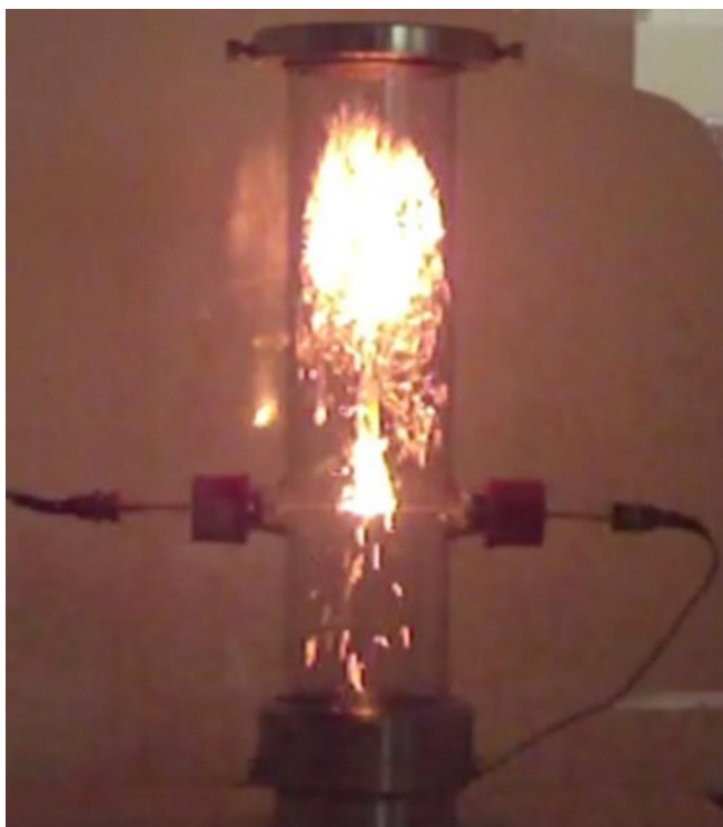
Explosion testing of carbon nanotubes
