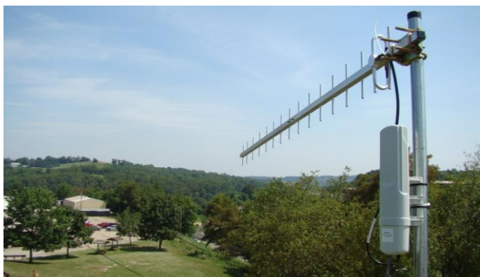
Figure 2. A Canopy™ Subscriber Module (SM) / Directional Antenna typically deployed at a remote site from the command center (CC).
