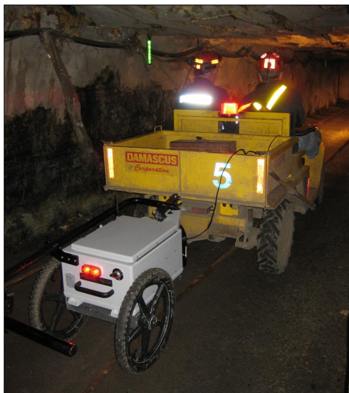
Figure 1. MineComms Mapper (MCM) being towed in a mine.
