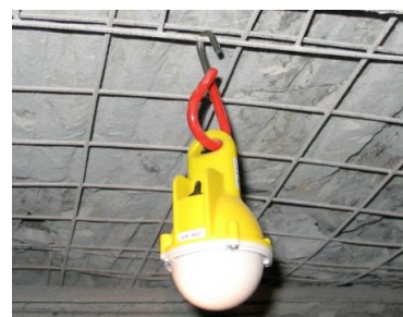
Figure 3. MSHA-approved UWB RFID tag with an estimated 10-year battery life.
