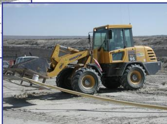
Moving dragline cable was one of the most physically demanding jobs performed. A J-hook bar is now used to drag the cable along the ground near the dragline. This eliminated the need to manually lift the cable. Away from the dragline, no physical effort is needed as the job now uses a cable-handling device attached to a front-end loader.
