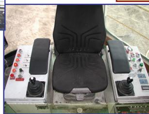
Dragline operators were complaining of upper-extremity discomfort and pain. It was determined that the support and function of the manufacturer-installed armrests were inadequate and nonadjustable. The new armrests were adjustable and provided larger nonfrictional support.
