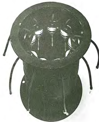
(d) Oblique view of aerosol sampling section with cyclones and collection filters in place
