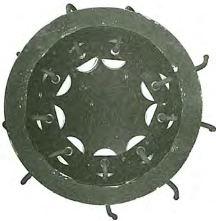
(c) Top view of aerosol sampling section with cyclones and collection filters in place
