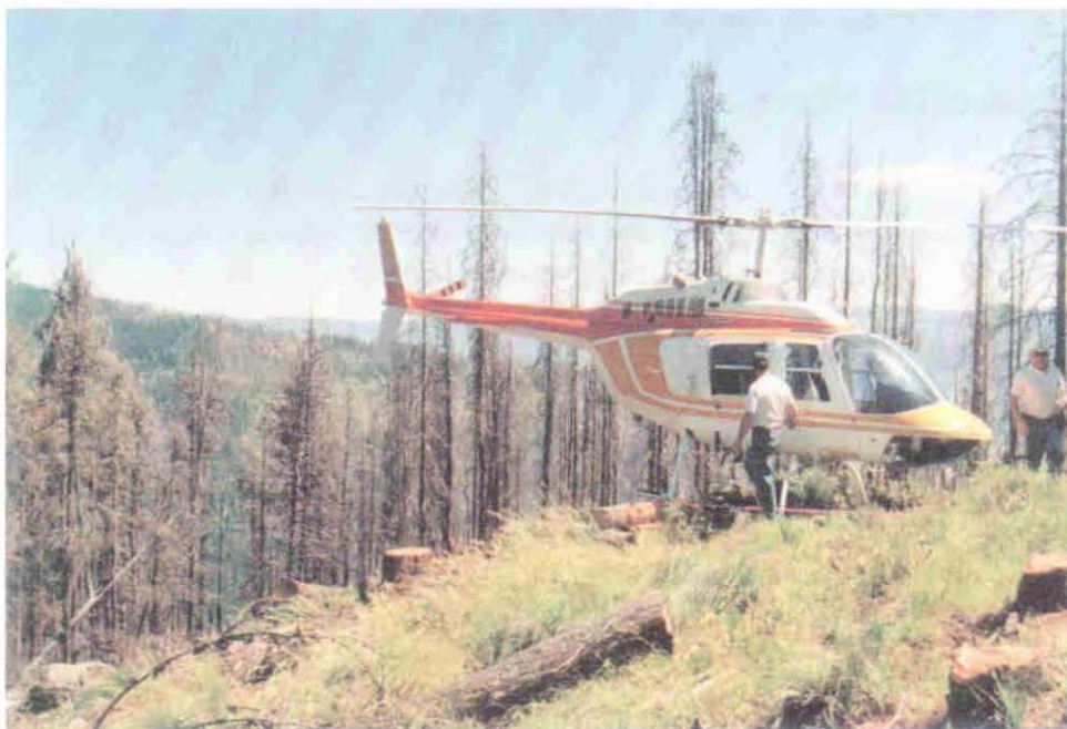
Photo 8. An example of a platform built on a steeply sloping bench. Pilots flying to these platforms contend with uphill rotor clearance, favorable landing conditions considering winds, and passenger safety when leaving and boarding.
