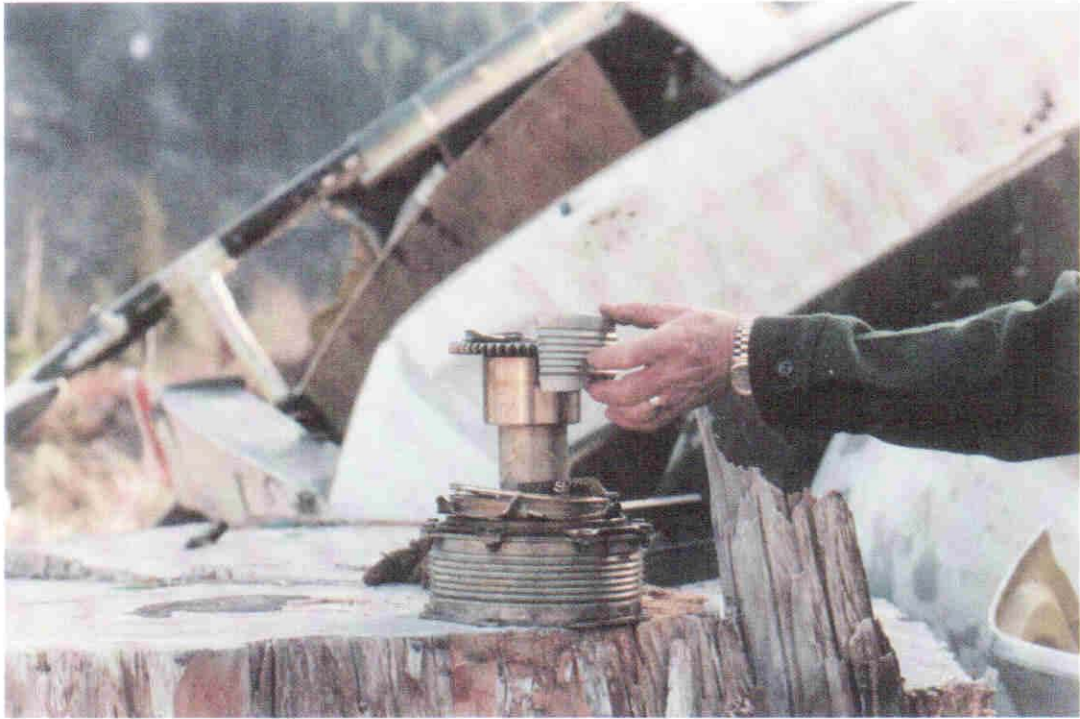
Figure 8. Drive Shaft and Rear Coupling Separated.
