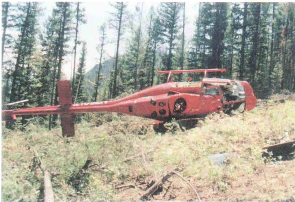
Photo 5. The Bell 206 rests on its right side, with it's main rotor separated at the mast. The left forward cockpit structure compromised by downward and rearward energy at the door frame from the broken blade. The tail cone and tail rotor showed neither damage nor pre-impact stoppage.
