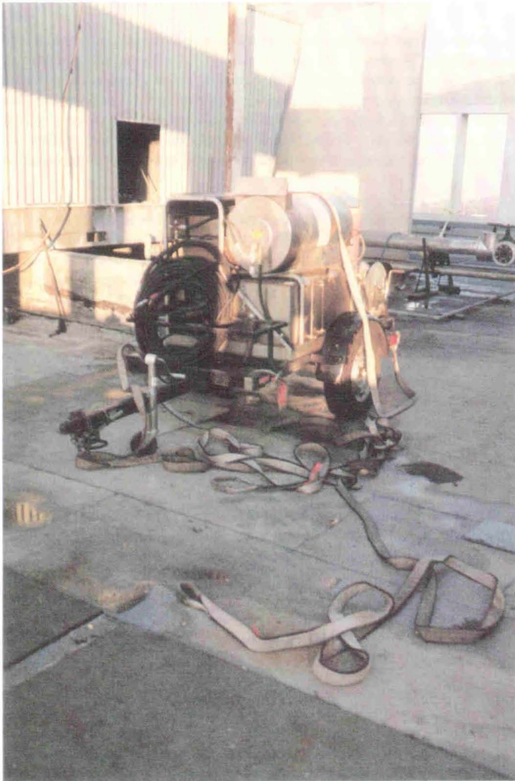
Photo 1. A steam cleaner, 100 foot long-line cable and lifting slings, set below the location of the dual engine power loss.
