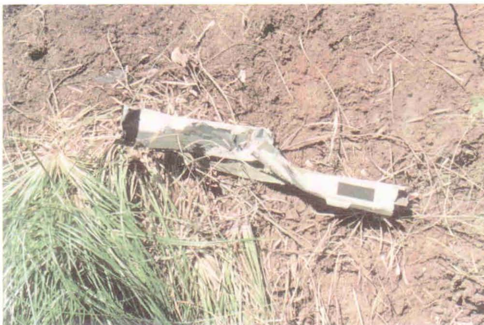
Photo 6. Left cockpit door post structure showing blade impact crushing.
