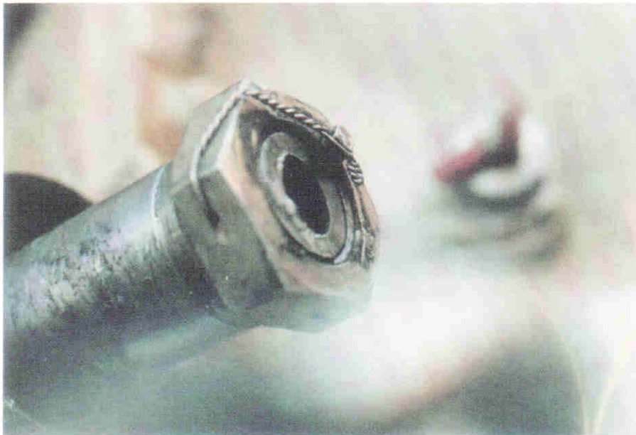
Figure 9. Location of Break on Right Cyclic Piston Rod.
