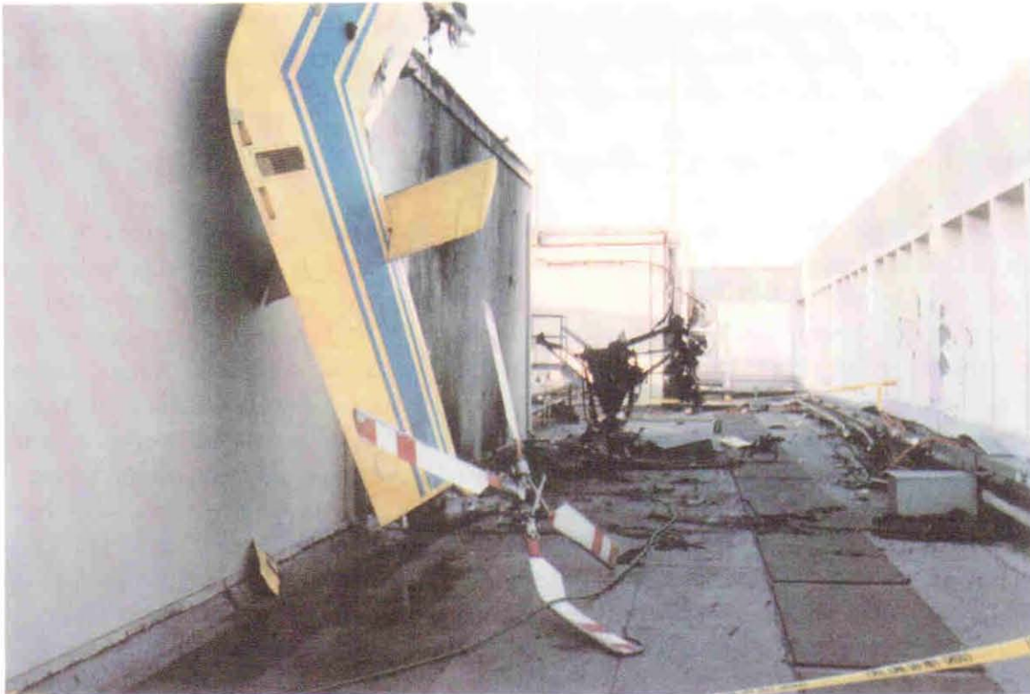
Photo 2. Wreckage of tail cone and tail rotor on the 13 th story roof of the building in downtown San Jose, January 28, 1994.
