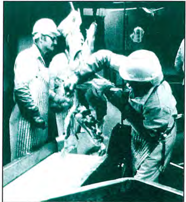
In a meat processing plant, working at a fast pace in cold environments while using forceful motions in awkward postures places individuals at risk for musculoskeletal disorders of the upper extremities.
