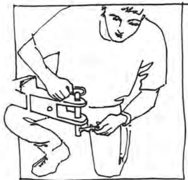
2-4. Secure all hitch pins with locking pins or clips. Consider using safety chains for road travel. Don't take the chance that the load could become unhitched.
