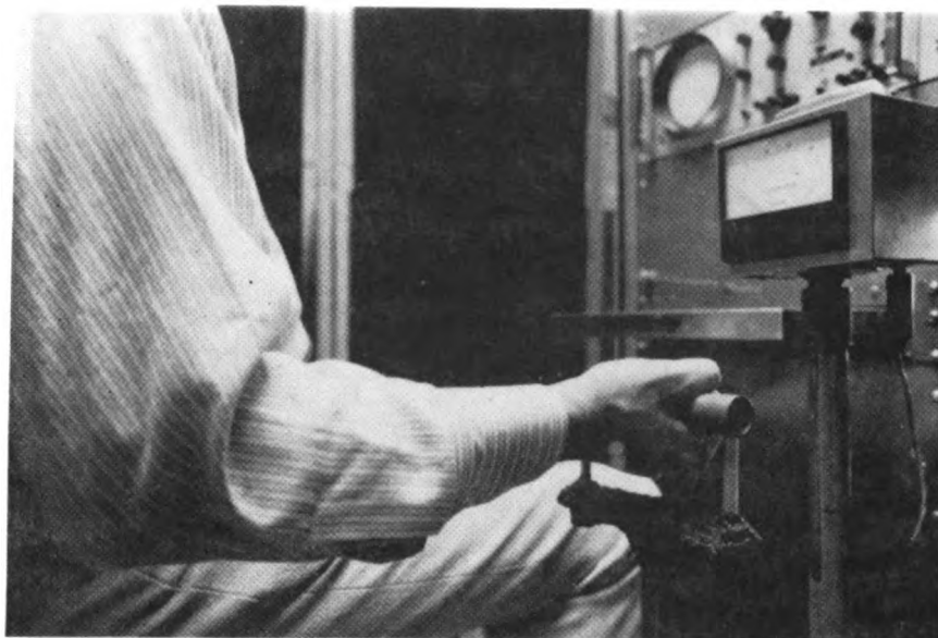
Figure 5. View of arm position during the test of strength (SER); both the handgrip dynamometer and subject display meter can be seen in this illustration.
