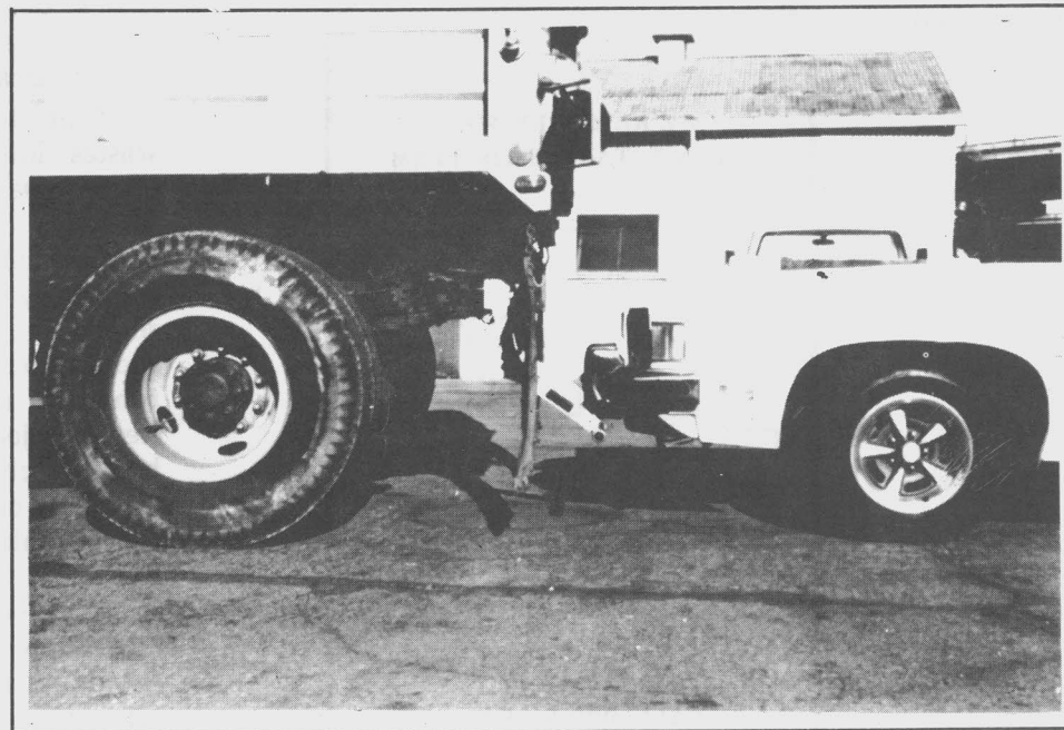
Figure 17. Pressure-sensitive backup safety device.
