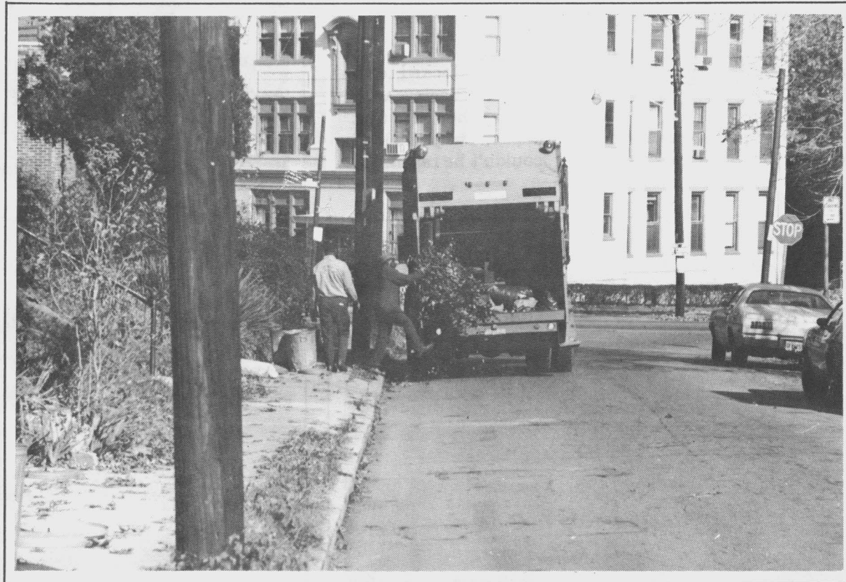
Figure 34. When truck is on left side of street, packer controls are on the traffic side.
