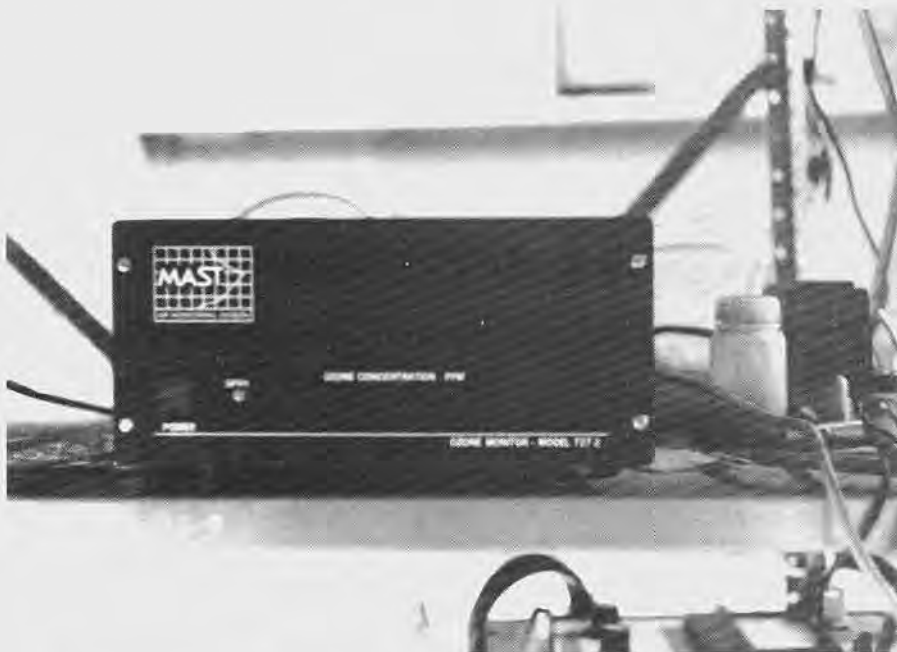
Figure 50. Photograph of Ultraviolet Ozone Monitor installed for testing.
