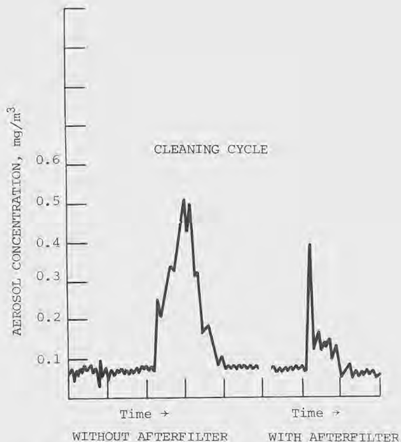
Figure 28. Aspirated Cartridge Filter - typical exhaust air aerosol concentration during cleaning cycle, with and without afterfilter.
