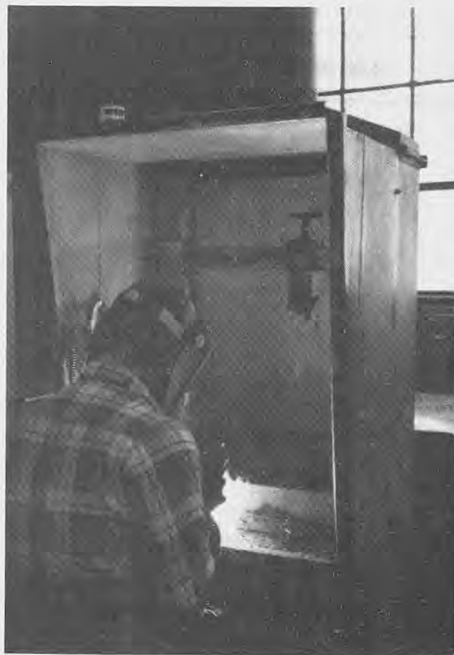
Figure 1. Typical welding operation within the ventilated booth.
