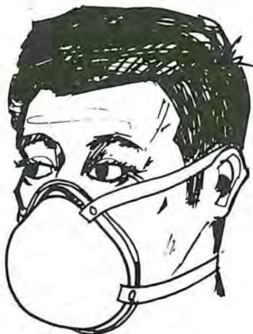
Side view showing proper position of straps
