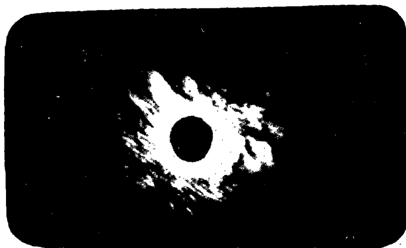
FIG. 19 Scattering Pattern from Amorphous Particle.
