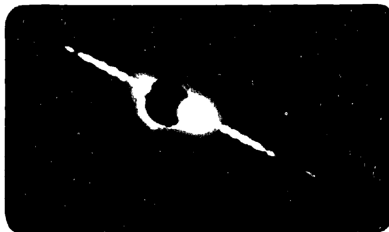
FIG. 21 Scattering Pattern From Stage Micrometer Line.
