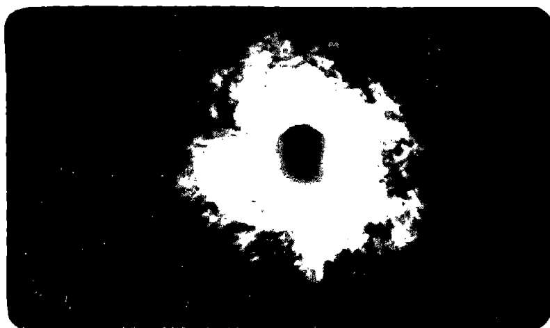
FIG. 18 Scattering Pattern from Amorphous Particle.
