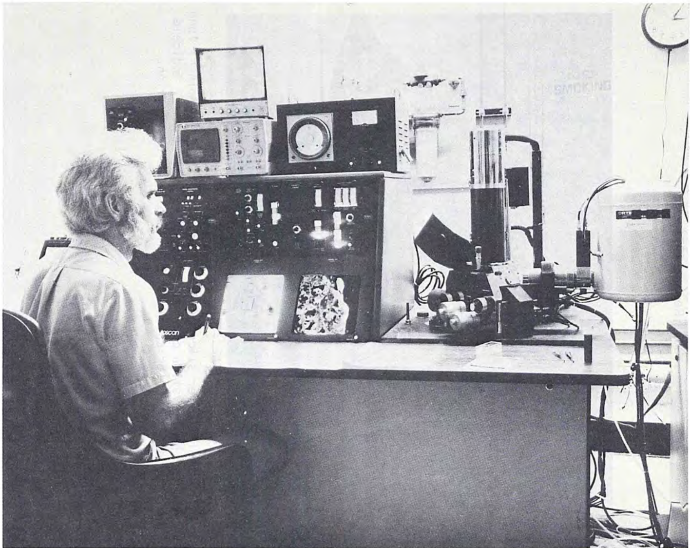
Figure 10. Scanning electron microscope being used to study CWP. Its high resolution and ability to analyze respirable dust particles make the instrument ideally suited for this type of research.
