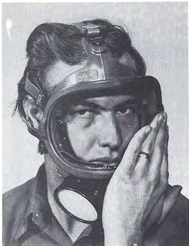
Figure 8-2. Positive pressure test.
