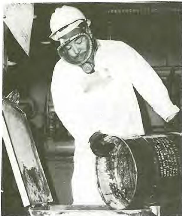
Figure 5-19. Typical chin style gas mask in use in a chemical plant.
