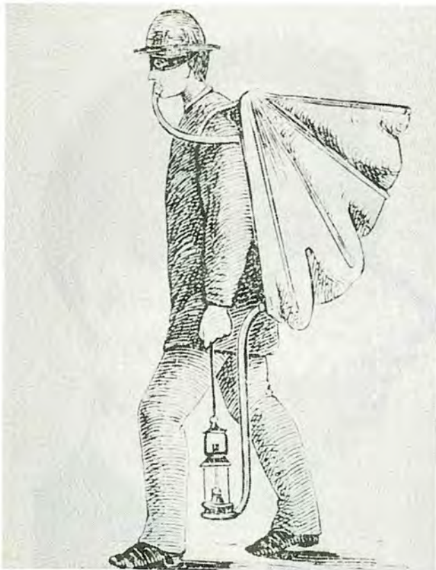
Figure 2-4. Magirus, Germany, ca 1840. Early positive pressure self-contained breathing apparatus.
