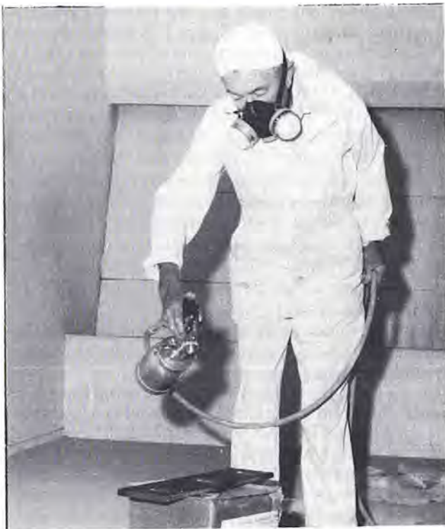
Figure 5-22. Typical combination particulate- and gas- and vapor-removing cartridge respirator being used in paint spraying.
