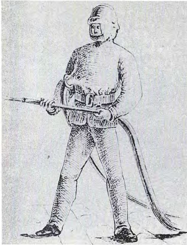
Figure 2-6. Magirus, Germany, ca 1820. Supplied air suit for firemen, similar to today's hose mask or air-line respirator.
