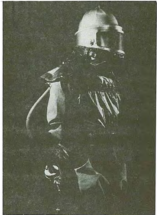
Figure 5-38. Supplied air hood for lead grinding. (Courtesy Mine Safety Appliances Co.)
