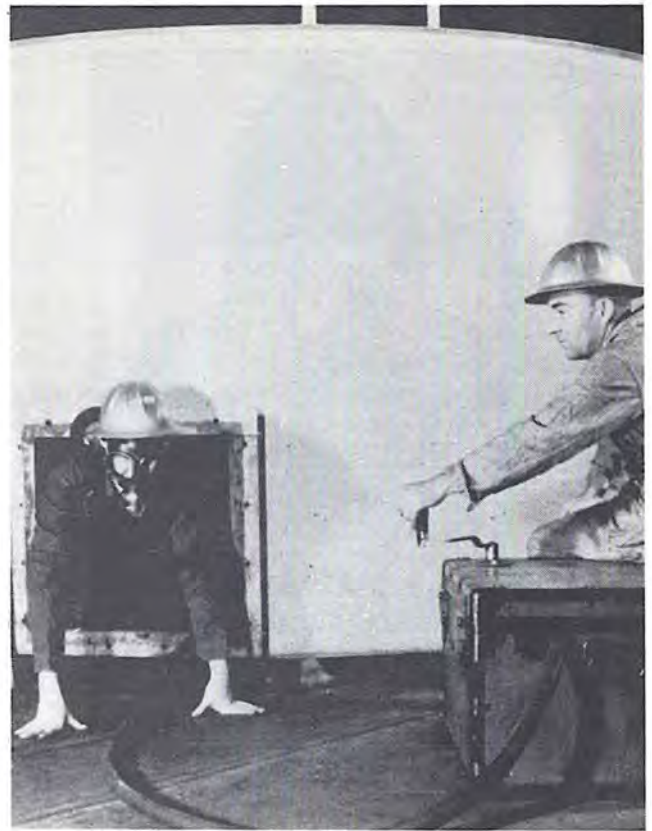
Figure 5-43. Typical hose mask with hand-operated blower being used for tank entry. (Courtesy Mine En- forcement Safety Administration.)
