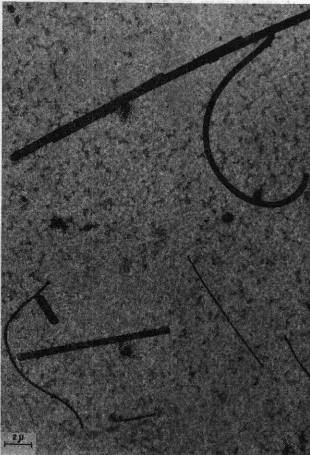
FIGURE 10-6. ELECTRON MICROGRAPH OF AIRBORNE FIBERS IN A SMALL FIBER PRODUCTION FACILITY
