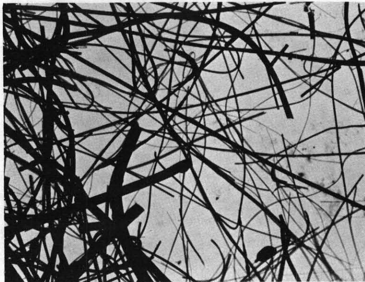
FIGURE 13-1. ELECTRON MICROGRAPH OF FIBERS SEVERAL HUNDRED MICRONS IN LENGTH WITH AVERAGE FIBER DIAMETER OF 0.05\ (\mu) MAGNIFICATION X 10,000
