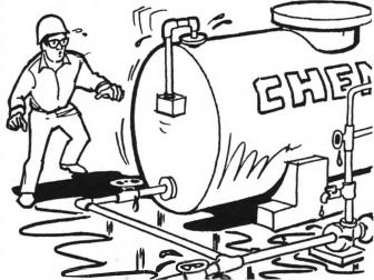
It's a good idea to make a dike ahead of time around pumps or other spots where you think a leak may occur so that leaks can be kept from spreading. If all the pumps can be kept in one area, it is easier to keep any leaks from spreading and to control vapors.
