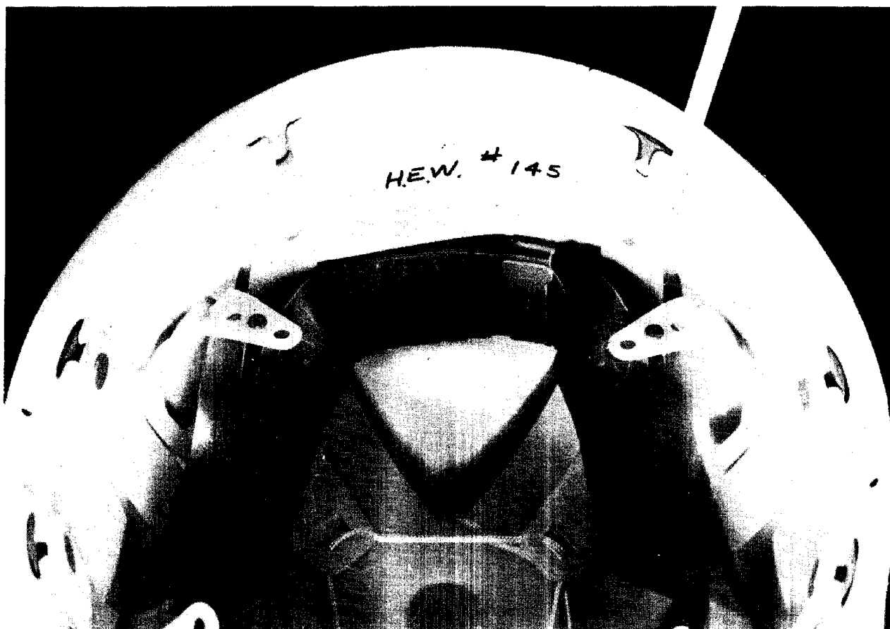
Photo. 14. Post shock absorption test, suspension mounting failure. Sample No. 145.
