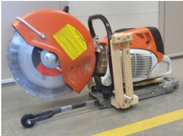
Figure 94. Final Design (Pull Springs not Pictured)
