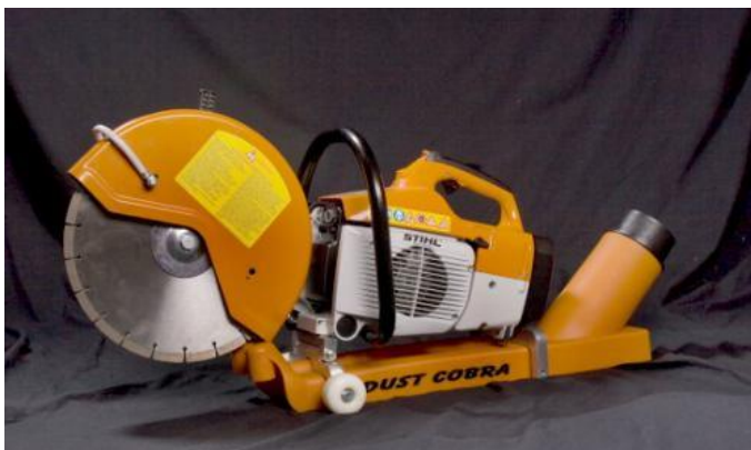
Figure 96: Dust Cobra Attached to STIHL Saw Used in Usability Testing
