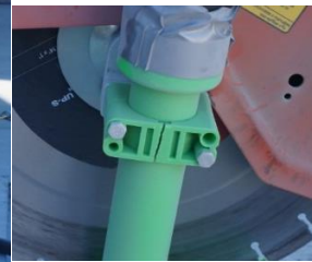
Figure 54. Cracked Saw Muzzle GP During Attachment
