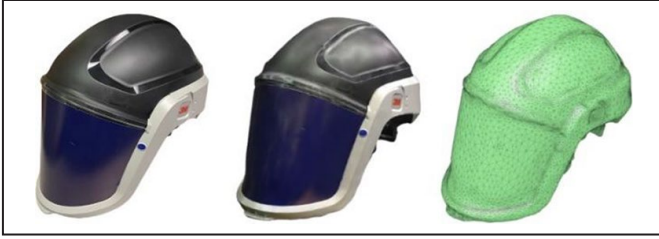
Figure 2. Real helmet (left), 3D points cloud (center), faceted body (right)
