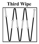
Figure 2. Wiping pattern for spiked tiles: Tiles were spiked and wiped using a three-pass method—W, Z, W.
