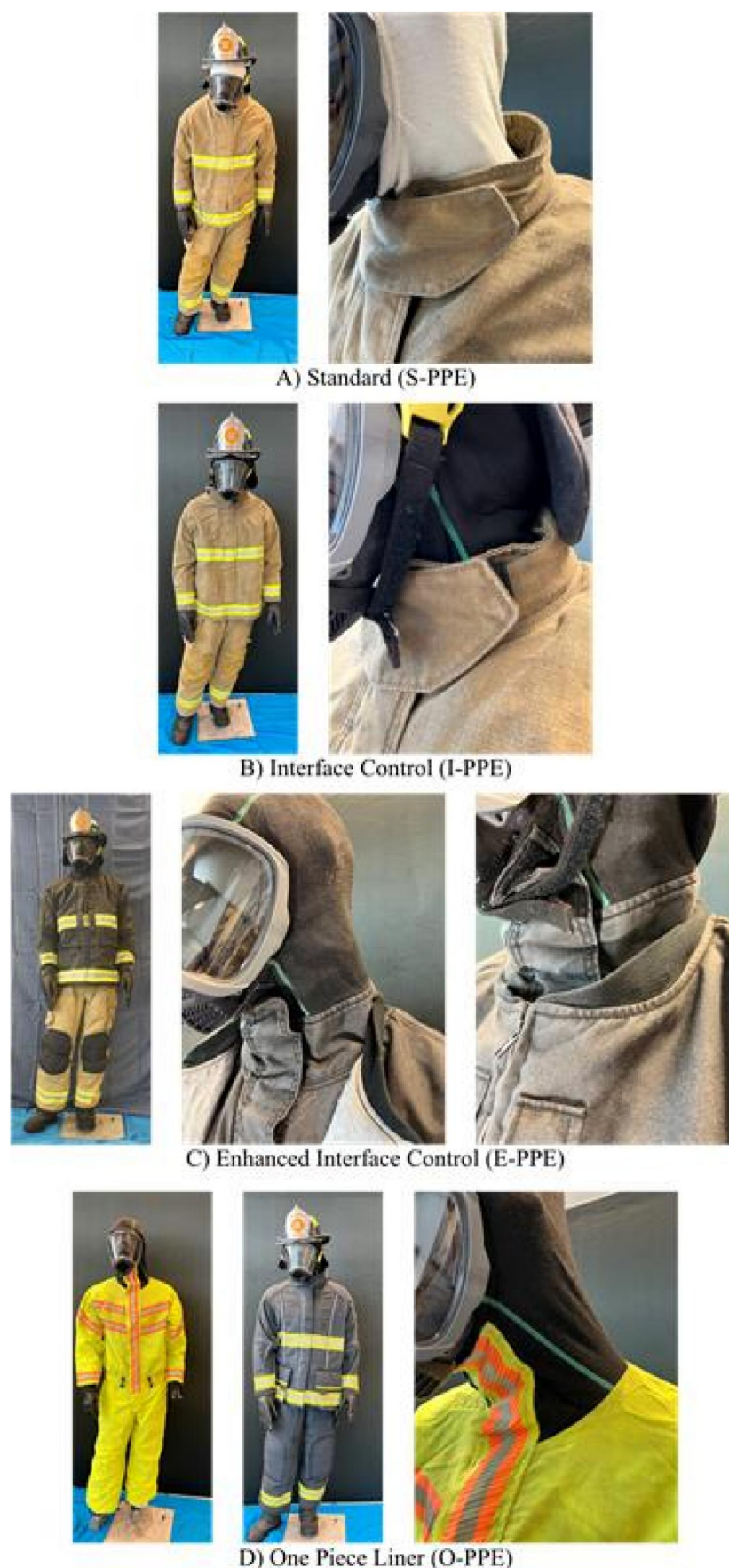
Figure 2. PPE conditions with increasing levels of interface control measures with hood involvement and mannequins: (A) standard (S-PPE), (B) interface control (I-PPE), (C) enhanced interface control (E-PPE), and (D) one-piece liner (O-PPE). All conditions were worn with cotton base layers before and after fire scenarios.
