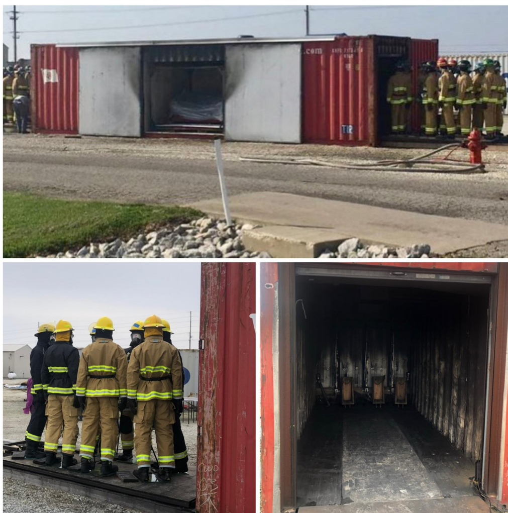
Figure 1. Fireground exposure simulator with mannequins dressed and prepared for smoke exposure scenarios. Mannequins are dressed in one of the four PPE conditions with varying and increasing contamination control measures.
