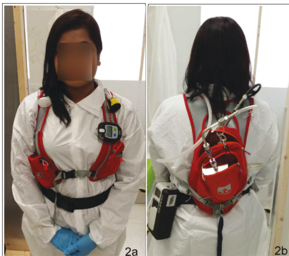
Figure 2. Home care aide wearing air sampling equipment to assess respiratory exposures while she performs cleaning in the residential bathroom built in the university environmental monitoring laboratory. Front (2a) and back (2b) views.
