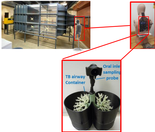
FIGURE 2: Experimental setup showcasing a custom-built dust wind tunnel with an integrated aerosol generator used to simulate the deposition of dust particles in the respiratory system.
