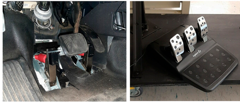
Figure 8. Integration and modification of the pedals with the Logitech G29 gaming controller.
