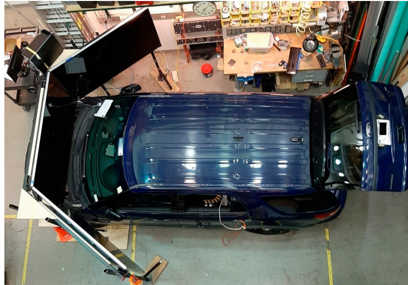
Figure 2. System setup of the virtual environment using a Ford Police Interceptor Utility in a lab setting.
