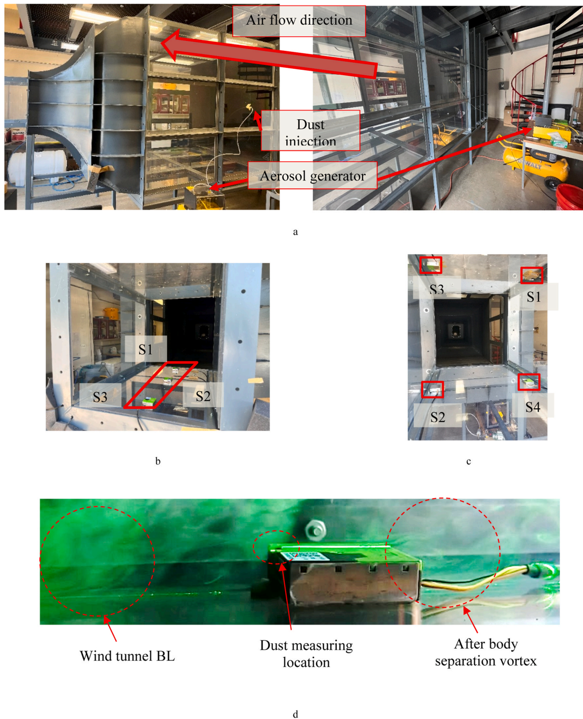
Fig. 11. Performance Validation Instruments: A comprehensive view of the integrated aerosol generator at the dust injection section, the strategically placed dust sensors in both linear and circumferential configurations.
