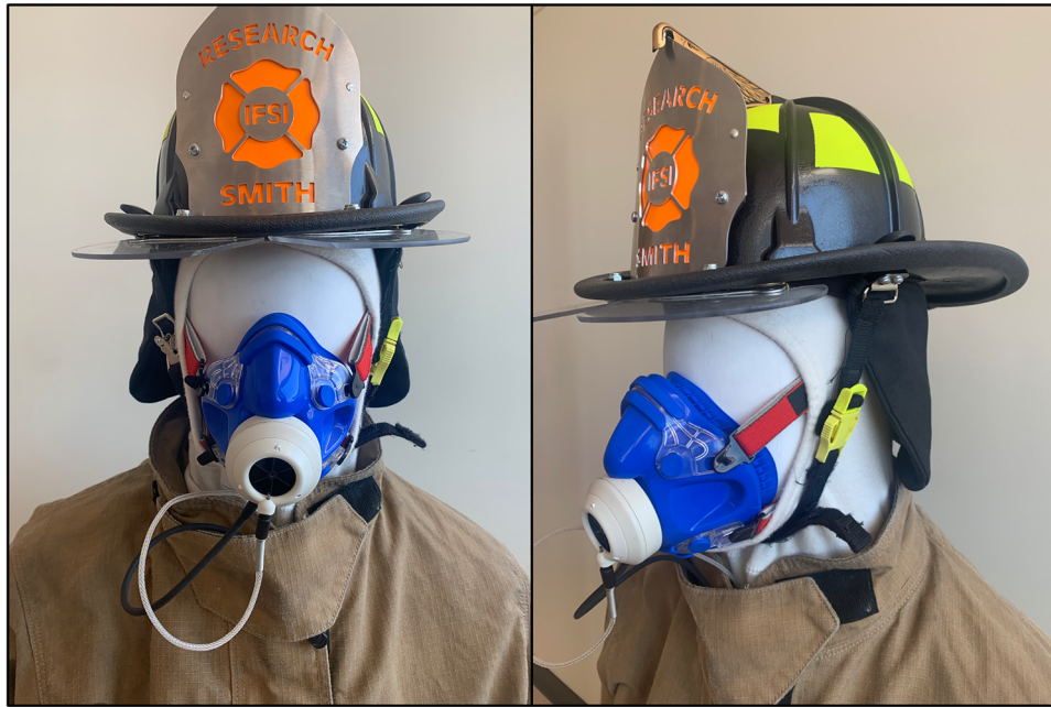
Figure 4. Participants wore the silicone K4b 2 metabolic monitor mask under the hood and helmet during firefighting activities.
