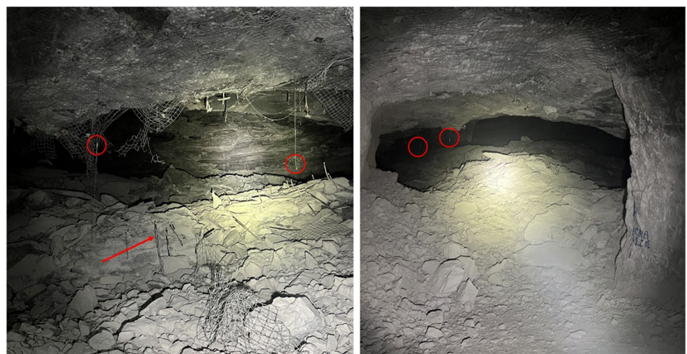
Fig. 8 Stope condition immediately after pillar removal. The red arrow indicates failed friction bolts noted in the stope. Red circles indicate locations where the fiber optic cable was severed between measurement boreholes
