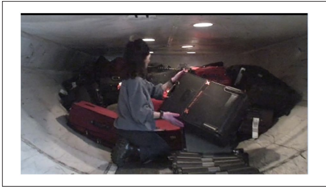
Figure 2. The portion of the Power Stow Rollertrack Conveyor (PSRC) is extended to the inside of the cargo hold of a narrow bodied aircraft (credit: NIOSH).
