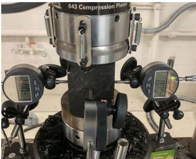
Fig. 5. Representative image from the coal sample deformability and UCS tests.
