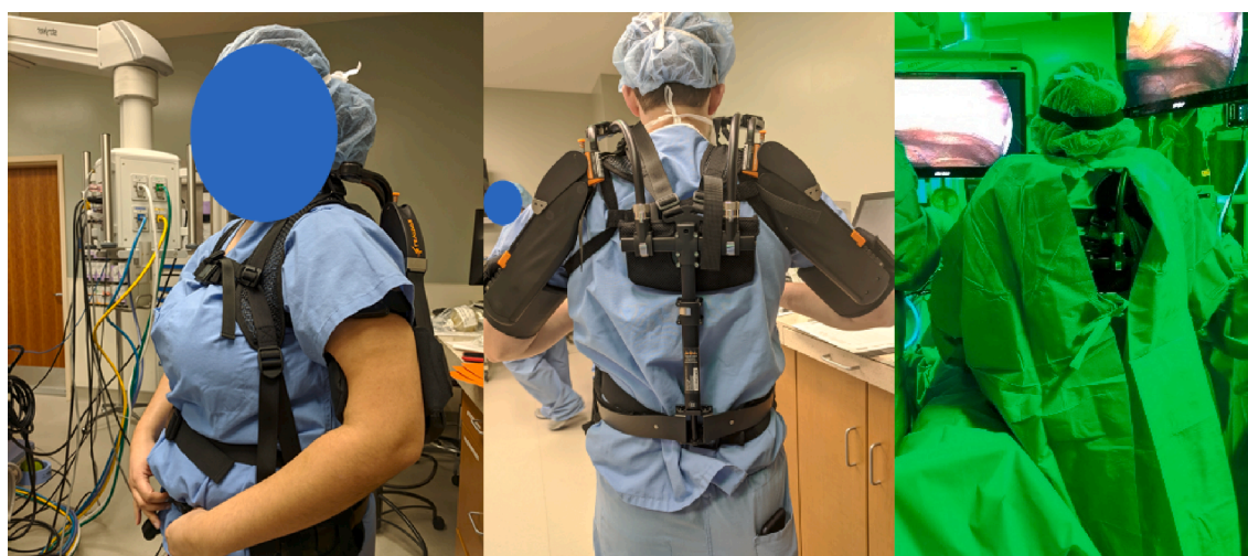
Fig. 1. Participant wearing the exoskeleton before surgery (left), a demonstration of how arms can be supported (middle), and a participant wearing the exoskeleton under a sterile gown during surgery (right).
