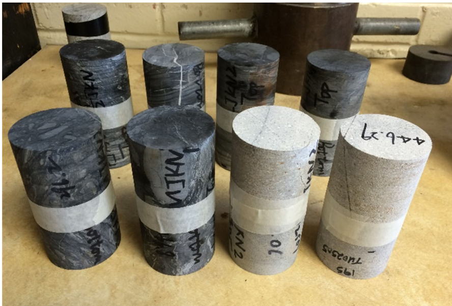
Fig. 2 Samples prepared for uniaxial compression test to estimate joint normal stiffness
