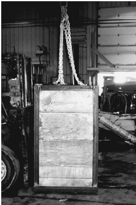
Fig. 7 Five-layered manufactured concrete block (Tang 2006)
