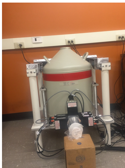
Figure 1. A photograph the four HPGe detectors. A Gd phantom is shown placed in front of the system.
