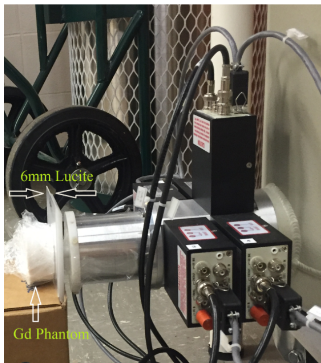
Figure 4. The 6.13 mm Lucite is shown placed between Gd phantom and detection system.
