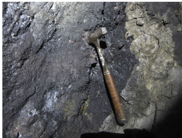
Fig. 16 Photograph of a weak rock mass with a Geo-Pick Strike Index (GPSI) of approximately one
