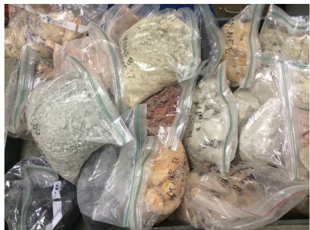
Fig. 11 Bulk samples of very weak rock taken from RMR mapped locations underground
