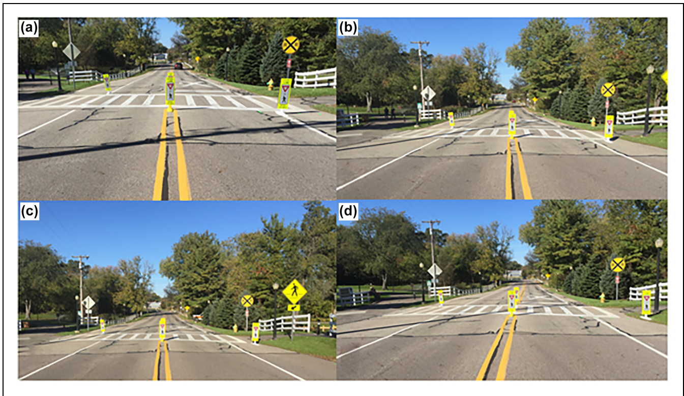
Figure 3. Gateway widths of (a) 12 ft, (b) 14 ft, (c) 16 ft, and (d) 18 ft.
