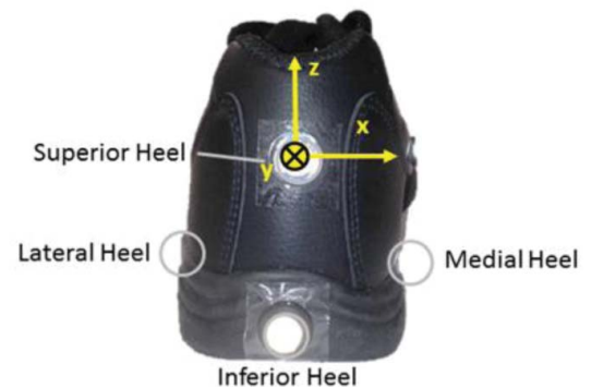
FIGURE 1 Reflective marker locations placed on the shoe from (A) top view and (B) posterior view.
