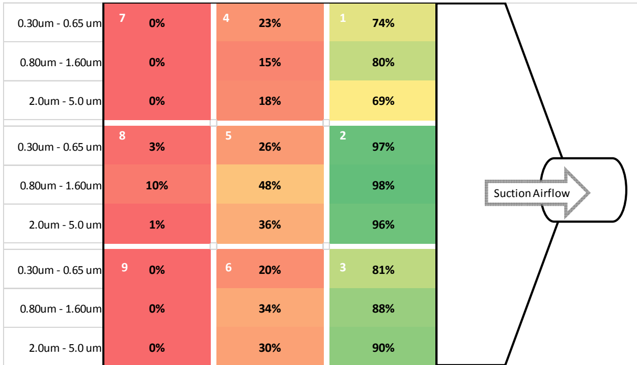
Figure 10: Collection efficiencies at 100 Lpm with plume velocity at 25 Ft/min.
