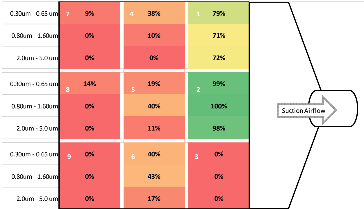
Figure 9: Collection efficiencies at 100 Lpm with plume velocity at 50 Ft/min.
