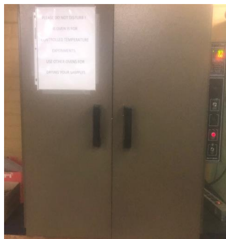
Convection oven at 100°C used to cure samples
