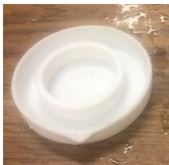
Teflon dishes (3-inch diameter and 0.6-inch-tall) and cylinders (2.1 inch diameter and 0.52-inch-tall) for casting samples
