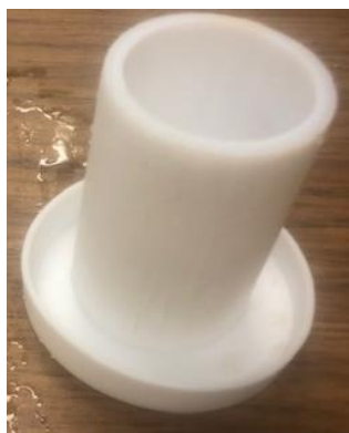
Teflon dishes (3-inch diameter and 0.6-inch-tall) and cylinders (2.1 inch diameter and 0.52-inch-tall) for casting samples
