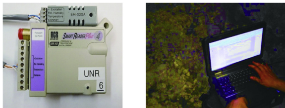
Fig. 5. Climatic data recorded by the monitoring units was downloaded on a laptop computer.
