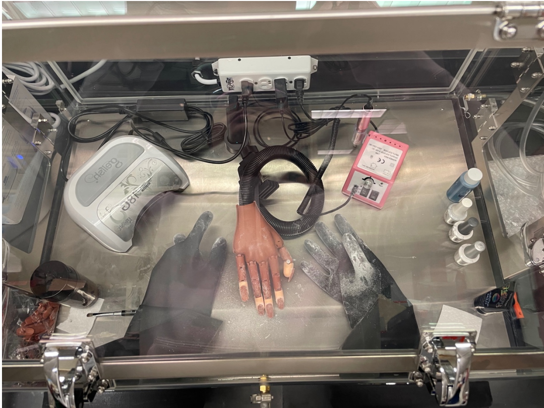
Figure 2. The setup of materials inside of the chamber. The port leading to the particle analyzers can be found in the bottom center of this image.
