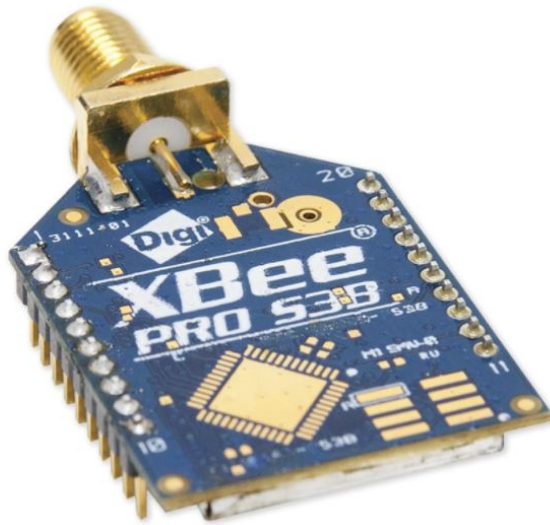
Figure D.7 Display of the XBEE Pro RF Module. Image from [106]
