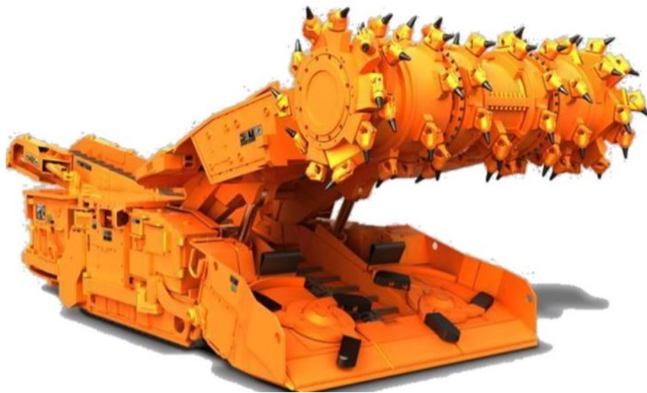
Figure B.1 Picture of a continuous mining machine which will serve as the basis for our dummy drum design. Image from [103]
