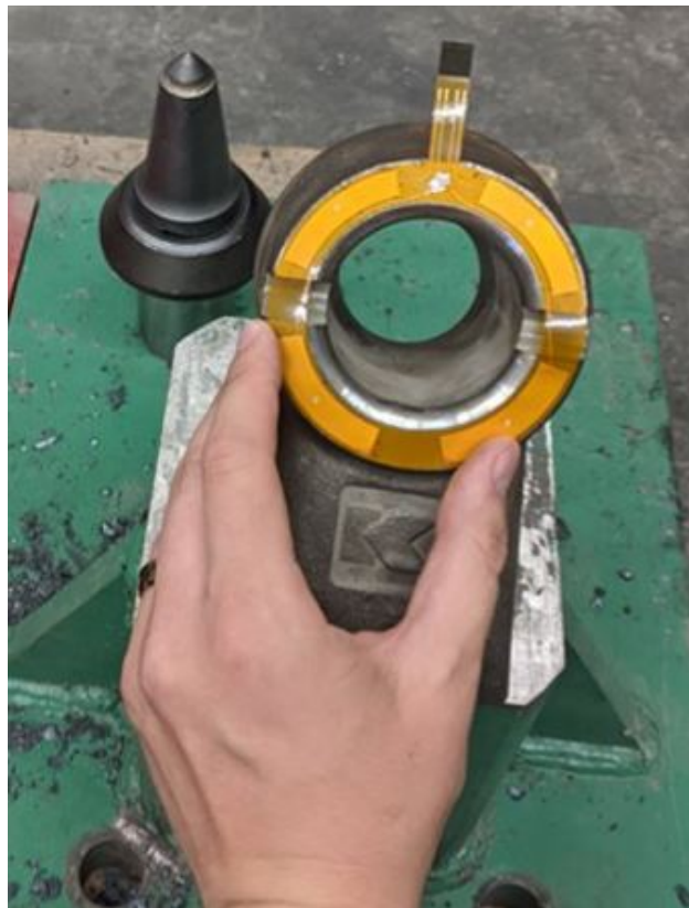
Figure D.1 Sensor configuration on the pick. The sensor we use has a total of four load cells
