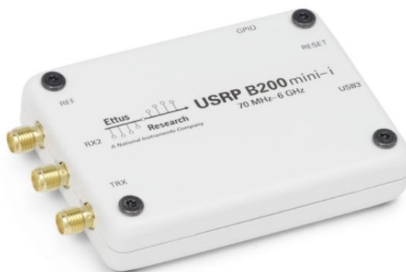
Figure D.2 Display of the b200 mini software defined radio. Image from [104]
