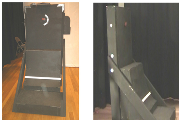
Fig. 4. Torque and push force measurement stands.
