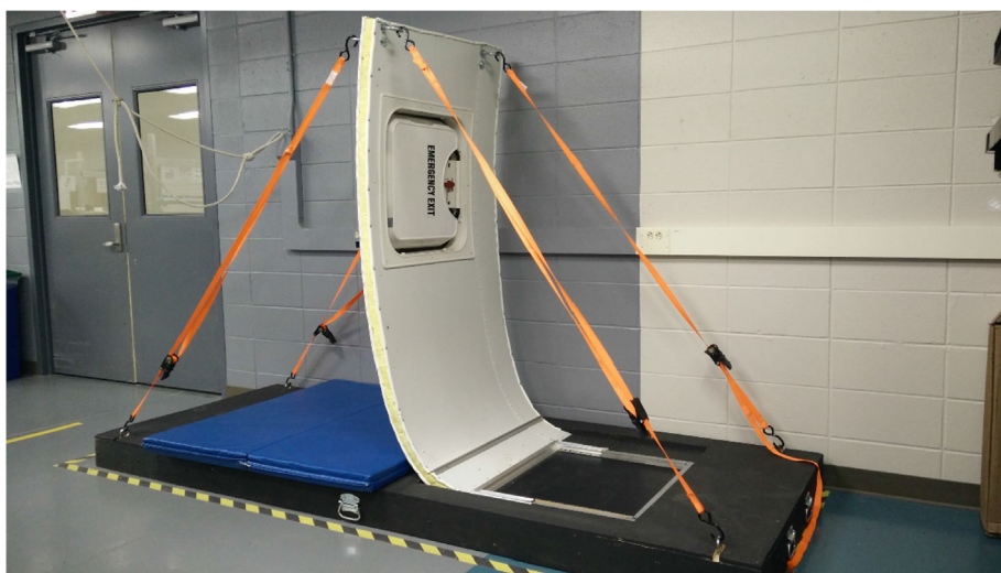
Fig. 2. Roof hatch evacuation test apparatus.
